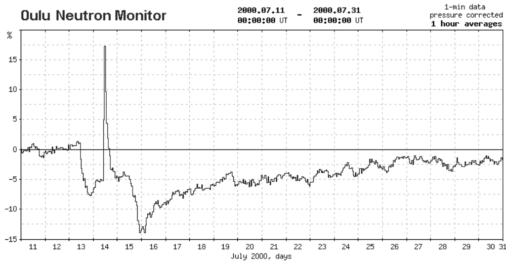
Figure 4: Neutron monitor count rate from the Oulu neutron monitor in Finland. A GLE was recorded on 14 July 2000, indicated by the sharp spike in the neutron monitor count rate (11:129).
